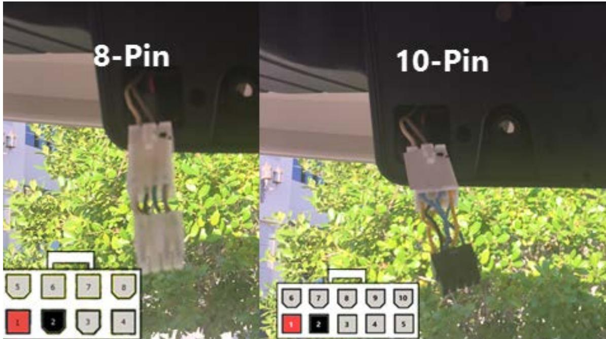
1. Use a number 2 or 3 Phillips hand driven screwdriver to remove the VDU from the console and expose the Molex connector.
