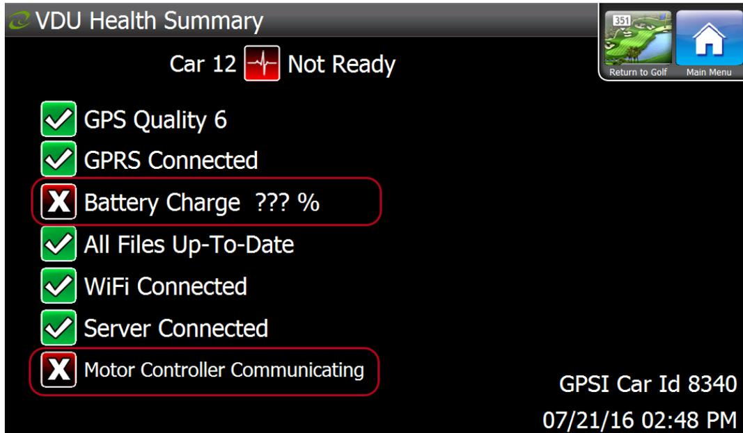
If the VDU and Motor Controller are not communicating, use the Flow Chart and documentation to diagnose and repair the problem.
