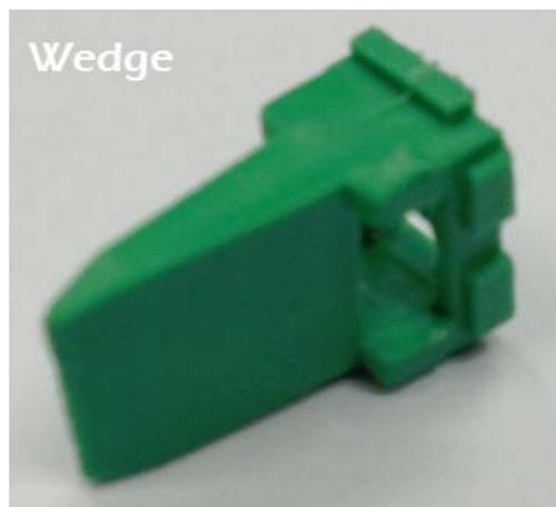
The replacement wedge can be installed by inserting the narrow end first, and locking it into place by pushing down with a small flathead screw driver or pick tool.
