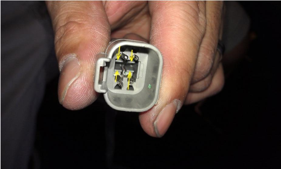
3. Make the appropriate pin adjustments using a pair of needle nose pliers and then reassemble the connector.
