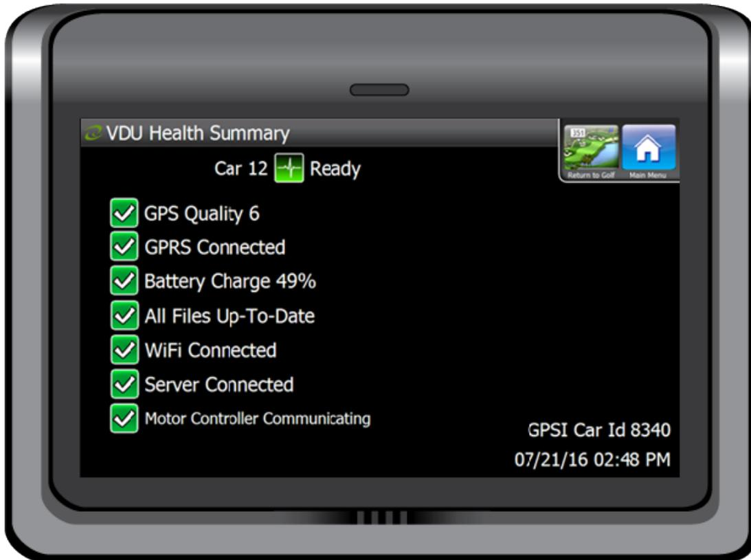
**If all of the previous components have been verified as functioning properly, the communication malfunction is somewhere in the motor controller, or supporting wiring and circuitry. A Club Car Factory Authorized Technician should be contacted to rectify the issue.**
