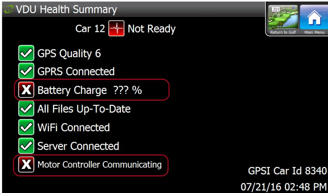
If the VDU to Motor Controller and / or OBC communications are not functioning properly, use the Flow Chart and documentation to diagnose and repair the problem.
