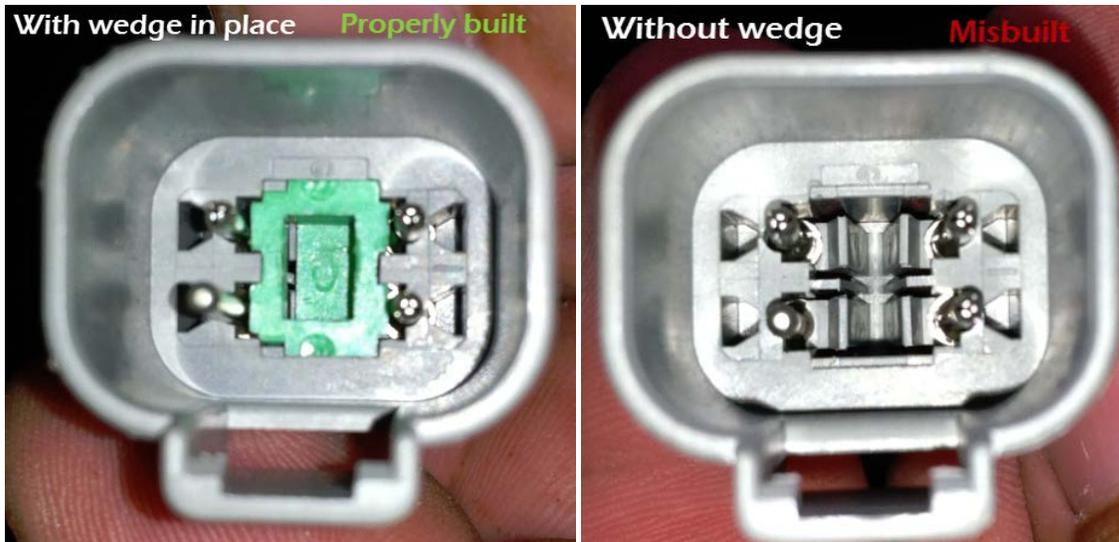
If the Deutsch connector was misbuilt without the wedge in place, a replacement wedge can be ordered through the GPSi parts department. **DO NOT** order a replacement strut.
