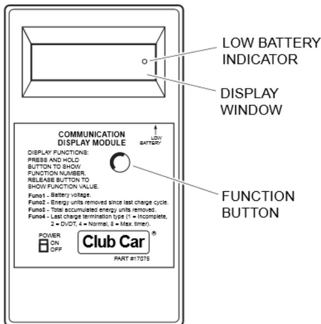
**STEP 1** – Using the POWER ON/OFF switch, turn the power ON.
