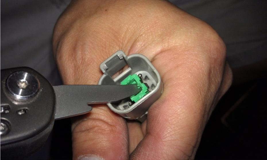
2. Once the wedge has been removed, you will see the clips which lock the pins into position. Move the tab away from the pin to release it, and towards the pin to lock it into position.
