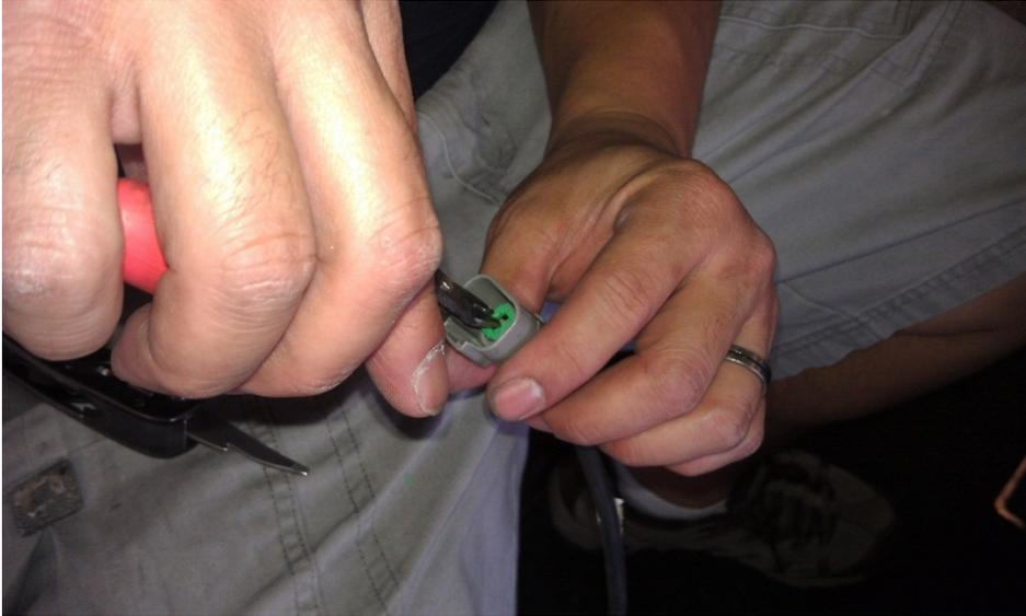
4. The wedge should be flush with the base of the connector, and the pins should all be fully extended.
