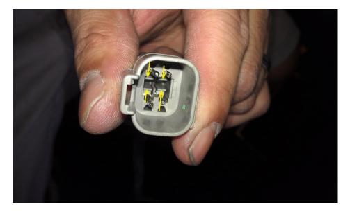
3. Make the appropriate pin adjustments using a pair of needle nose plyers and then reassemble the connector.
