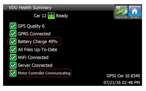
• A VDU that is not communicating with the car will display a red box with an "X' next to Motor Controller Communicating and Battery Charge % field.
