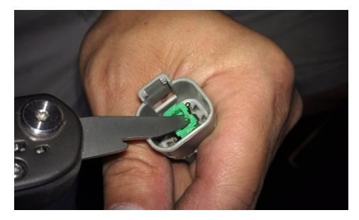
2. Once the wedge has been removed, you will see the clips which lock the pins into position. Move the tab away from the pin to release it, and towards the pin to lock it into postion.
